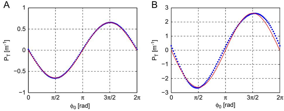
**Fig. 3.** Transverse focusing power ( $P_T$ ) versus phase offset ( $\phi_0$ ) for field amplitudes  $E_0=0.5$  MV/m (A) and  $E_0=2$  MV/m (B). The theoretical values are indicated by the red solid curve and the simulated values by blue dots. (For interpretation of the references to color in this figure caption, the reader is referred to the web version of this article.)
