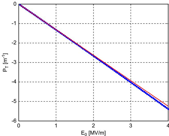
**Fig. 5.** Transverse focusing power ( $P_T$ ) versus field amplitude ( $E_0$ ) for a fixed phase offset  $\phi_0=\pi/2$ . The theoretical values are indicated by the red solid curve and the simulated values by blue dots. (For interpretation of the references to color in this figure caption, the reader is referred to the web version of this article.)
