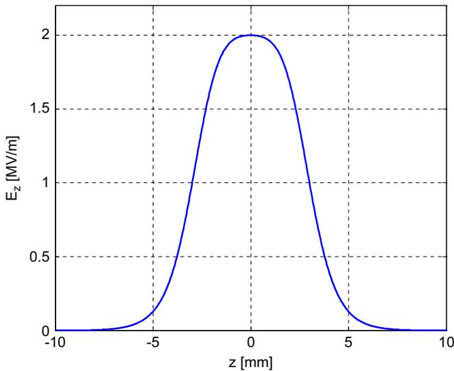
Fig. 1. The  $TM_{010}$  field profile used in the simulations. For this field profile, the effective cavity length  $d_c=6$  mm.
