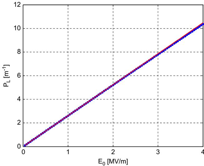
**Fig. 4.** Longitudinal focusing power ( $P_L$ ) versus field amplitude ( $E_0$ ) for a fixed phase offset  $\phi_0=\pi/2$ . The theoretical values are indicated by the red solid curve and the simulated values by blue dots. (For interpretation of the references to color in this figure caption, the reader is referred to the web version of this article.)
