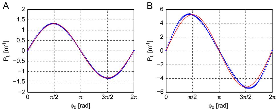
Fig. 2. Longitudinal focusing power ( $P_L$ ) versus phase offset ( $\varphi_0$ ) for field amplitudes  $E_0=0.5$  MV/m (A) and  $E_0=2$  MV/m (B). The theoretical values are indicated by the red solid curve and the simulated values by blue dots. (For interpretation of the references to color in this figure caption, the reader is referred to the web version of this article.)
